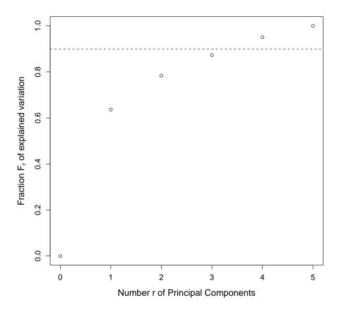
Since the first three PC's capture 87% of the variability, and the first four 95%, it is tempting to proceed with a reduced model with only r=3 or 4 variables. How will this affect the analysis?
