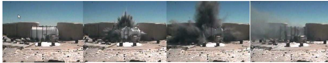
Figure 4: A modern implosion experiment carried out at the dual axis radiographic hydrodynamic test facility at LANL. High energy x-rays interrogate the object as it implodes.
