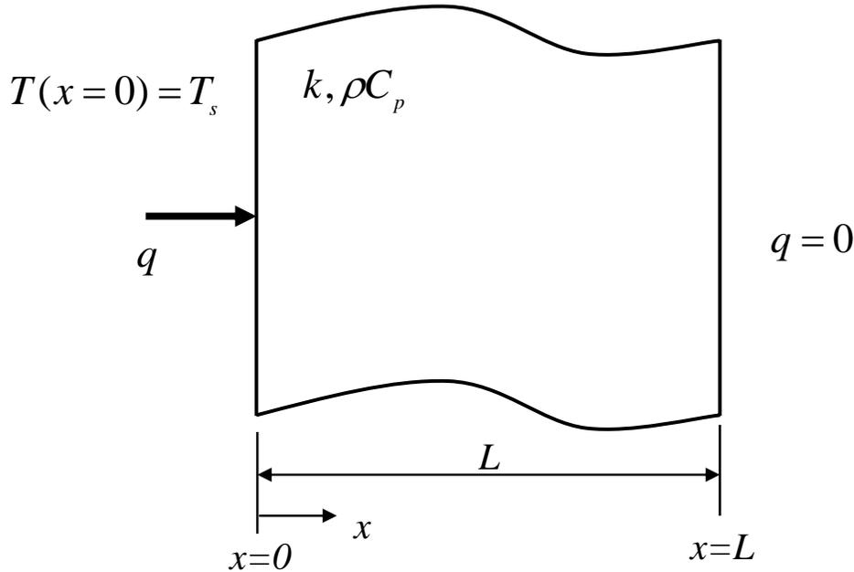
Figure 1. Schematic of heat conduction problem
