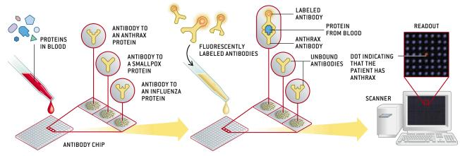
Apply blood from a patient to a chip, or array, consisting of antibodies assigned to specific squares on a grid. Each square includes multiple copies of an antibody able to bind to a specific protein from one organism and so represents a distinct disease-causing agent.
