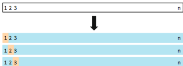
Figure 6: A set of n data points is repeatedly split into a training set (shown in blue) containing all but one observation, and a validation set that contains only that observation (shown in beige).
