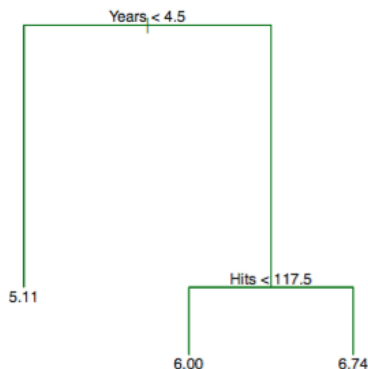
Figure 1: A regression tree for predicting the log salary of a baseball player, based on the number of years that he has played in the major leagues and the number of hits that he made in the previous year. At a given internal node, the label (of the form X_j < t_k ) indicates the left-hand branch resulting from that split, and the right-hand branch corresponds to X_j \geq t_k .
