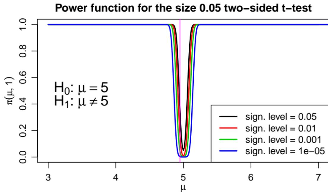
Power function for  $n = 1000$  for different  $\alpha_0$  levels.
